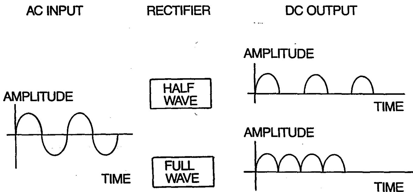
**Figure 3.4: Rectified Current**
